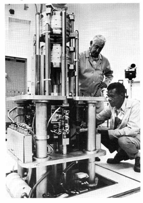
PULSE TESTING of SPR-III, fast burst reactor, is underway in Area V. Operators are J.C. Conant and Vern James (both 5421). Primary use of the new reactor will be tests of weapons and electronics packages. When not in use, SPR-III is lowered into shielded pit below the floor.
